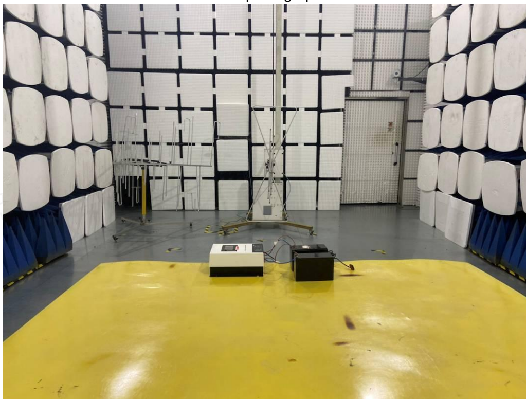
Test Setup Photo of Radiated Measurement (30MHz~1GHz)
